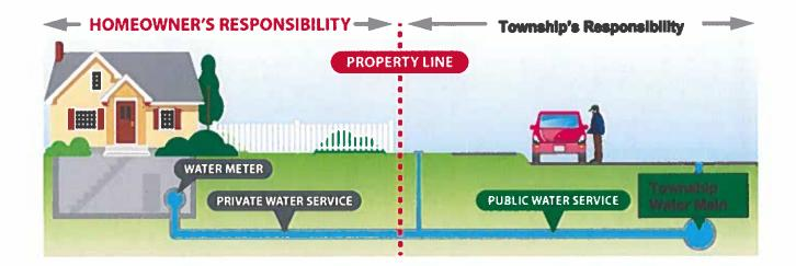
In most cases, the property line ends a few meters from the edge of the curb or sidewalk. The diagram above shows that the water service valve is placed very close to the property line, but it is not always on the Township's side, however the Township owns it.
